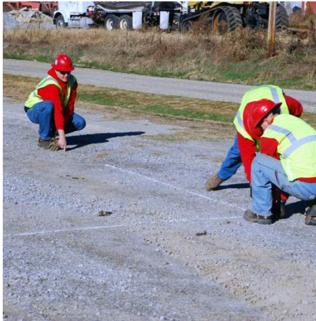
Step 1: Choose site that is flat and level twice the length of your longest truck
